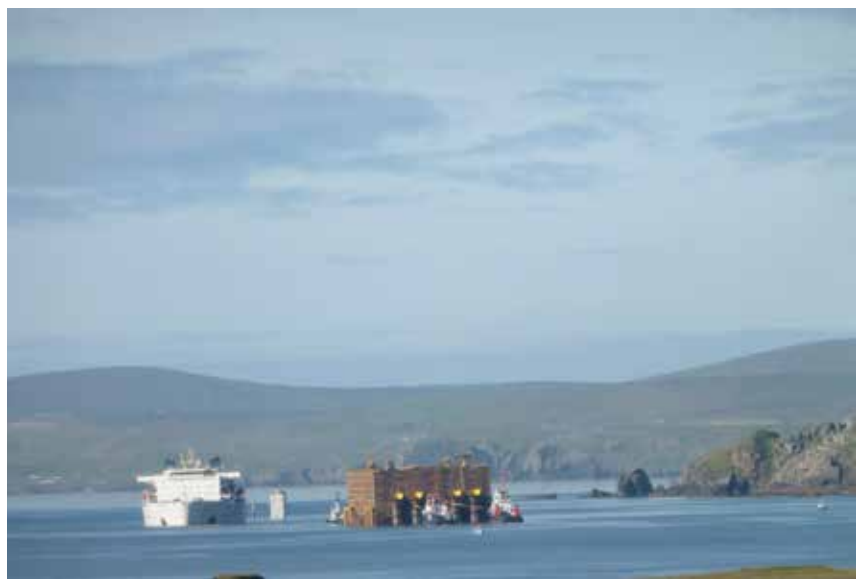
Chinese semi-submersible Xiang Yun Kuo, ballasted down to allow a large tank to float off its deck into the care of waiting tugs.
